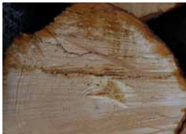
Maskinorsakade sprickor i al.
